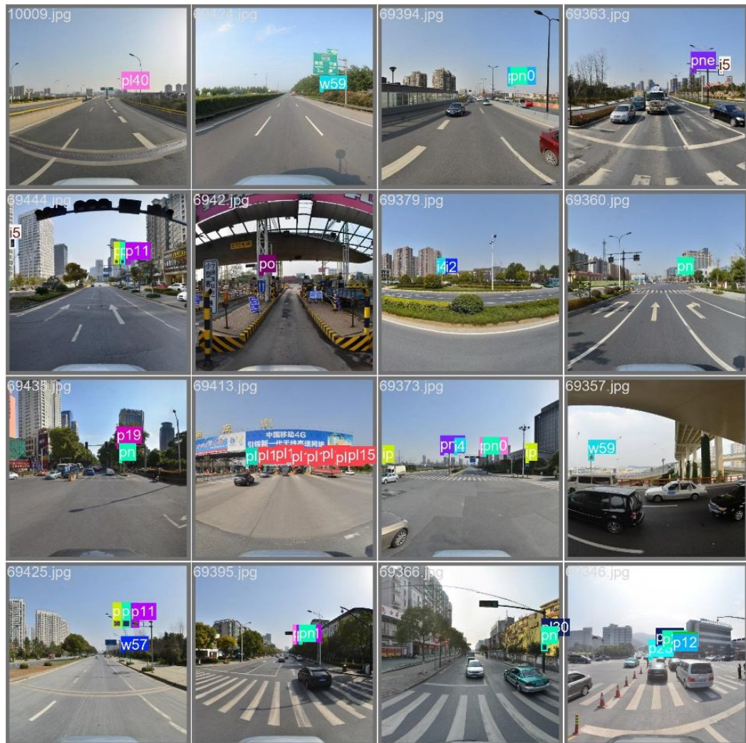
Fig. 15 (Part I). This image displays the recognition results for real road condition images or video data, with 'pl19' being one of the labels and 0.9 representing the probability of it being that label.
